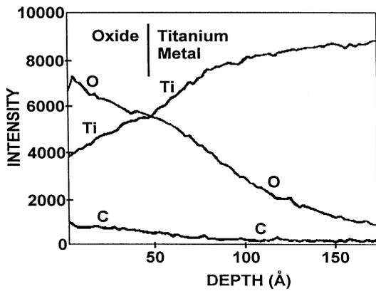
Fig. 5. AES depth profile of passivated titanium. The thickness of the oxide layer is relative to the sputtering rate of  $Ta_2O_5$ .
