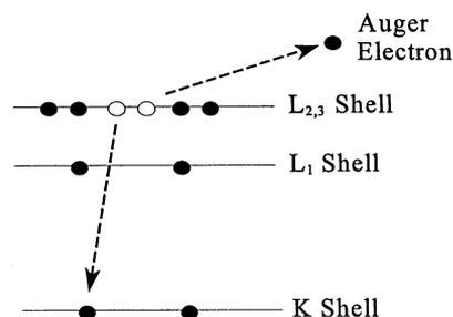
Fig. 2. Schematic showing the immediate de-excitation of the excited atom, resulting in the emission of an X-ray or Auger electron.
