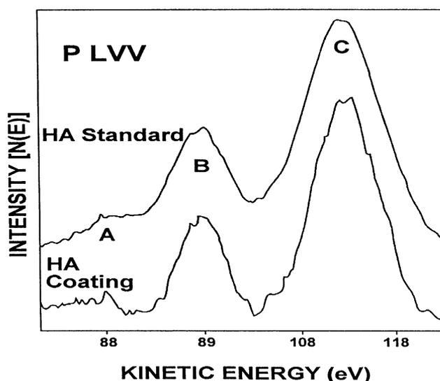
Fig. 11. PLVV  $N(E)$  surface spectra of HA standard and HA coatings. The kinetic energies A, B, and C correspond to the energies in Table 1.
