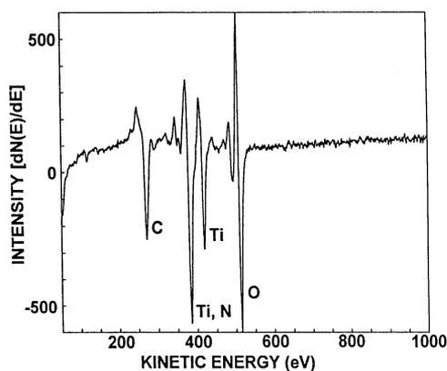
Fig. 10. Ti Auger derivative surface spectrum of passivated titanium showing a significant carbide buildup after long beam exposure. Overlap of the Ti and N peaks were also observed.
