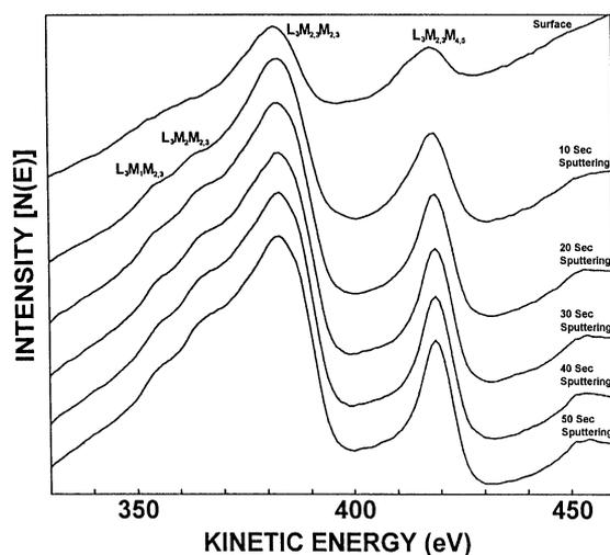
Fig. 7.  $Ti_{LMM} N(E)$  spectra of passivated titanium showing shape changes as a result of alternate sputtering and analysis cycles.
