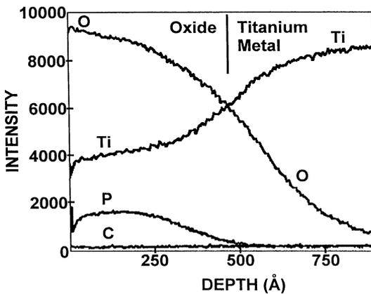
Fig. 6. AES depth profile of anodized titanium. The thickness of the oxide layer is relative to the sputtering rate of  $Ta_2O_5$ .
