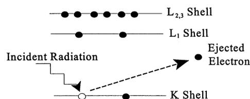
Fig. 1. Schematic showing the irradiation of the KLL shell. The interaction leaves the atom in an excited state with a core hole or a missing inner-shell electron.
