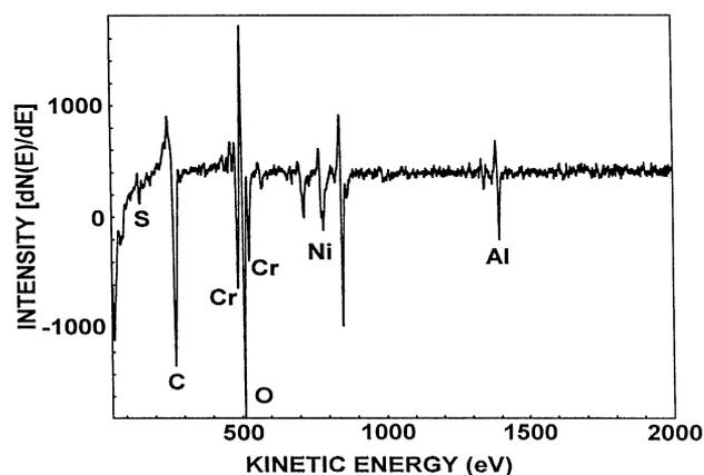
Fig. 4. Example of an AES spectrum showing a differential mode,  $dN(E)/dE$ , plot of Ni–Cr–Be dental alloy.
