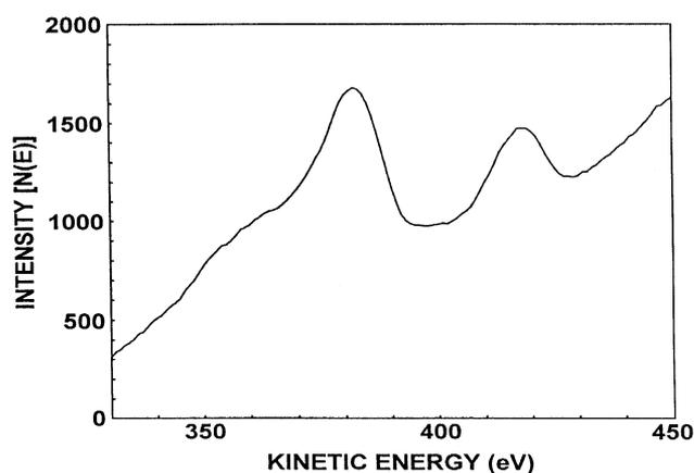
Fig. 3. Example of an AES spectrum showing a direct electron energy distribution,  $N(E)$ , plot of Ti LMM.
