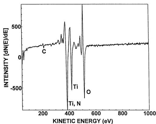
Fig. 9. Ti Auger derivative surface spectrum of passivated titanium showing a small carbide peak after minimal beam exposure.
