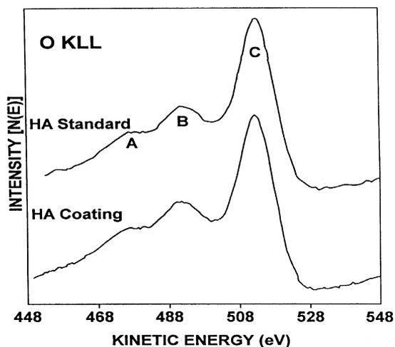
Fig. 12. OKLL  $N(E)$  surface spectra of HA standard and HA coatings. The kinetic energies, A, B, and C correspond to the energies in Table 1.
