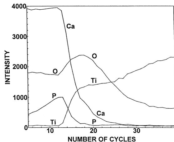
Fig. 8. AES depth profile of HA coatings showing the migration of phosphorus (P) during ion bombardment.
