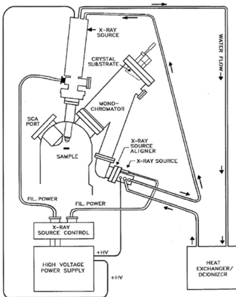
Figure 1-1. PHI Model 10-420 Toroidal Monochromator Package/System Interface.
