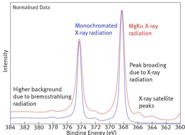
Comparison of Ag 3d spectra with monochromatic and non-monochromatic radiation (normalized to maximum peak intensity). Monochromatic peaks are cleaner and thinner.
