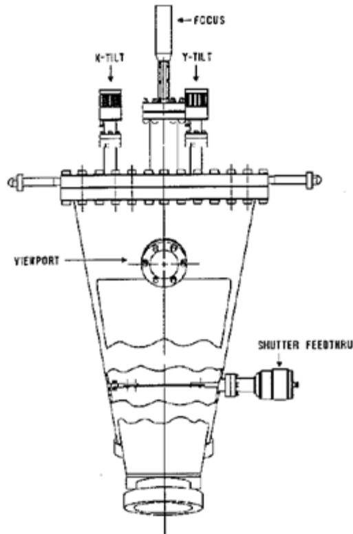
7. Position the silver specimen at the focal point of the analyzer and sputter to remove carbon and oxygen contamination. Adjust the specimen tilt angle to 45° (horizontal). Connect a picoammeter to measure target current.
