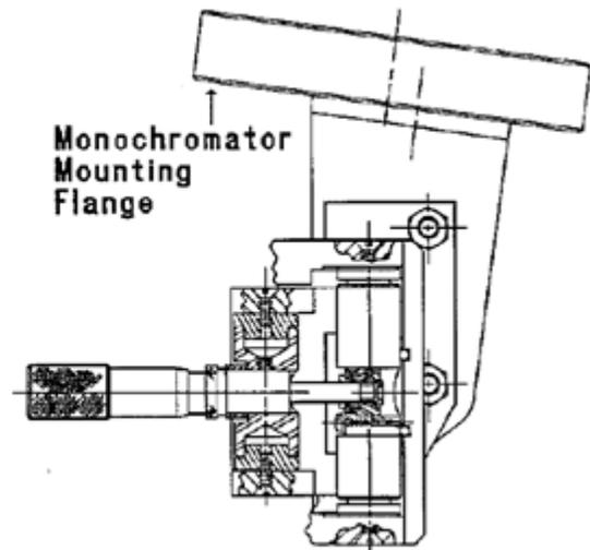
Figure 3 - 8. Right side view of x-ray source aligner.
