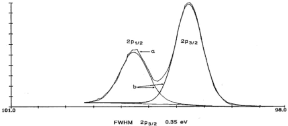
Figure 3 - 9. Data acquired on a Si wafer with the monochromator using a 1.1 mm dia. aperture and PSD detector. This Si 2p spectrum shows several advantages of the monochromator. Line a shows the raw data. Without the monochromator, the Si 2p doublet would appear as a single peak. Line b shows a curve fit of the raw data by two peaks.
