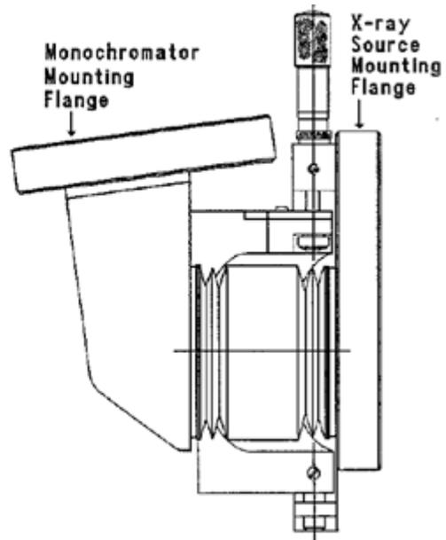
Figure 3 - 6. Left side view of x-ray source aligner.
