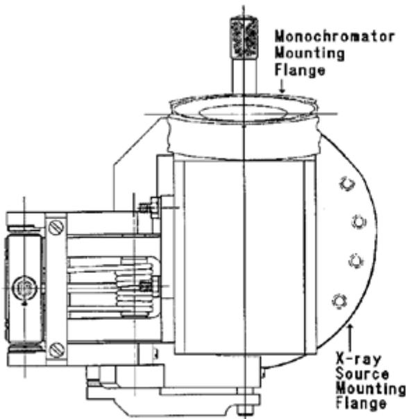
Figure 3 - 7. Rear view of x-ray source aligner.
